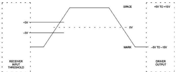
Figure 1. RS-232 Logic Level Specifications
