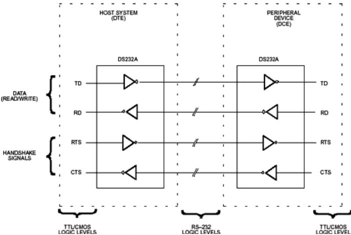
Figure 5. Half-Duplex Communication Scheme
