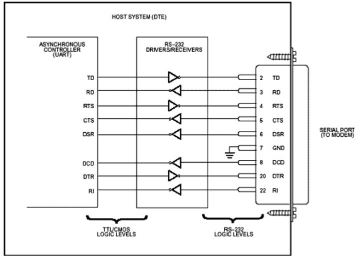
Figure 3. Typical RS-232 Modem Application
