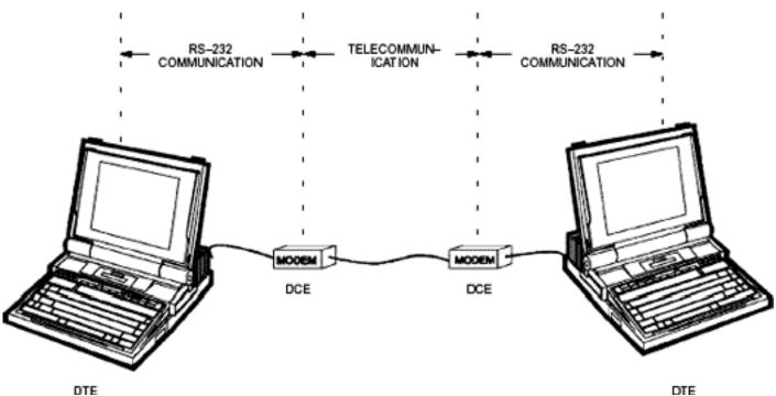
Figure 4. Modem Communication Between Two PC'S
